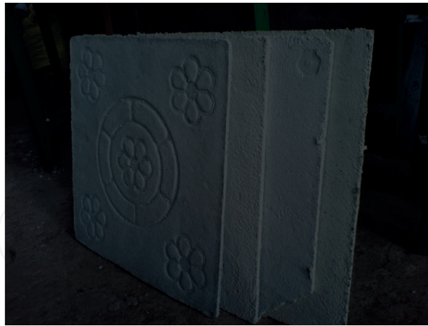
Figure 10. Made-in-Nigeria wastepaper-cement composite ceiling boards. Source: [16].
