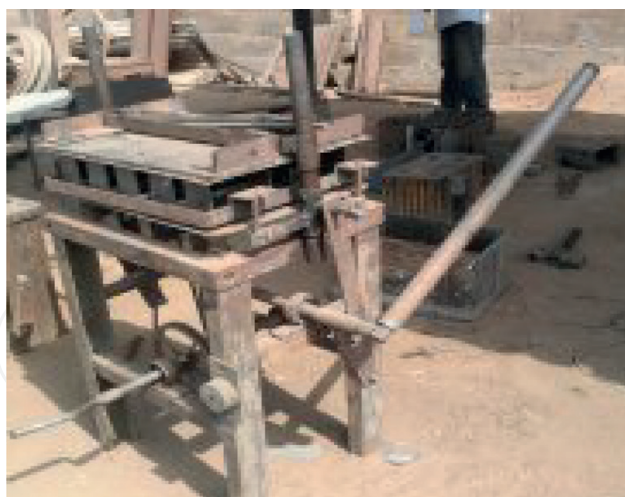
Figure 13. Side view of the tile-making machine. Source: [41].
