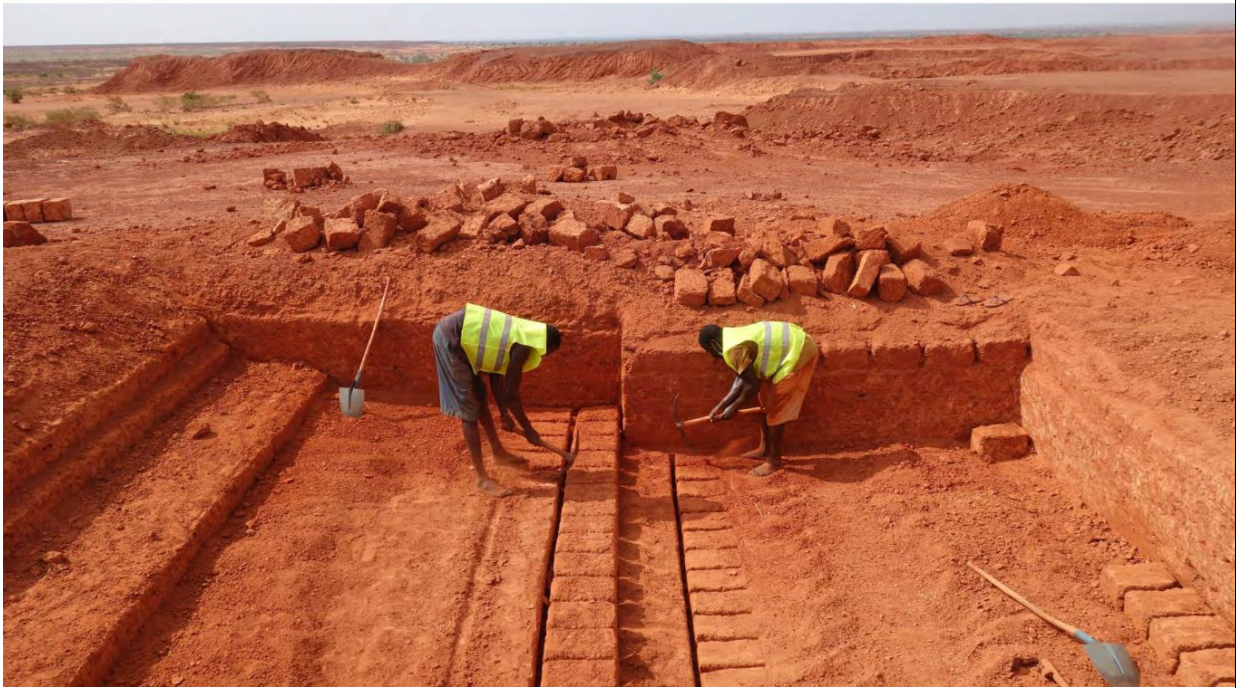
Digging up laterite from the ground in local quarry. Credit: Grant Smith
